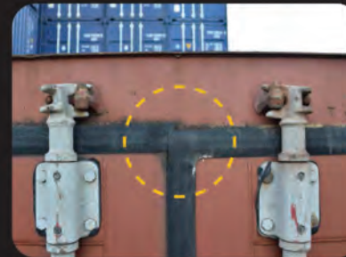
Container Not Level
